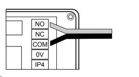
Ensure the wiring is neat and secure and fit the lid back to the box. 5. Connect the free end to the Mini Monitor and secure with the locking screws
