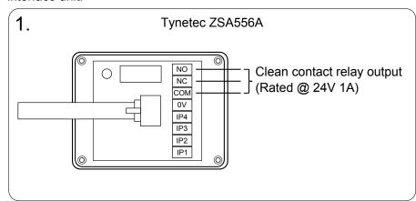
2. Connect a suitable length of twin core low voltage cable to terminals NO & COM of the Tynetec unit (shown here in grey and black).
