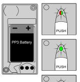
When a battery is first fitted the indicator light will flash red then green a few times.
